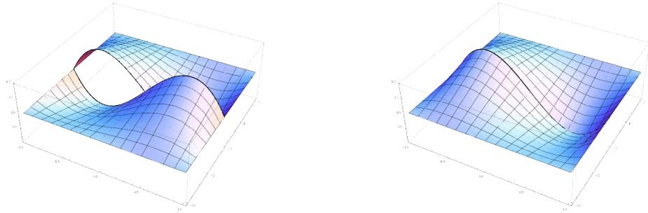
vertex, edge and cell based basis functions on reference element  $\hat{T}$ :
