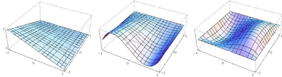
edge based basis function on two neighbouring quadrilateral elements without and with taking care of orientation:
