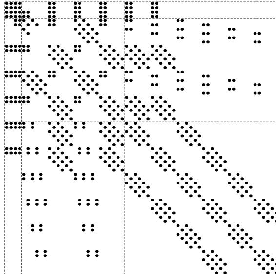
stiffness matrix entries for hierachic Legendre-type basis on the reference element  $[-1, 1]^2$ :
