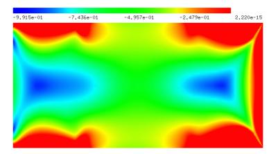
Figure 21: Yield function  $\phi$  (8) in Example 2.
