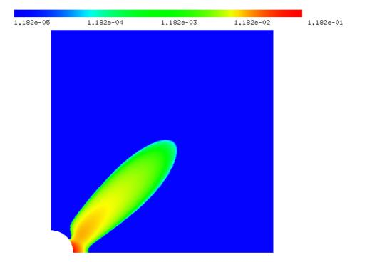
Figure 41: Logarithmic Frobenius norm of the plastic strain in Example 3.
