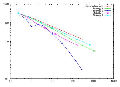
Figure 52: Here, the global estimated error (45) is plotted versus the time (in seconds) which was spent per Newton step in Example 3. One Newton step covers the assembling of the stiffness matrix and a sparse direct solver (PARDISO).
