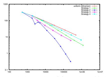
Figure 51: The global estimated error (45) versus degrees of freedom in Example 3.
