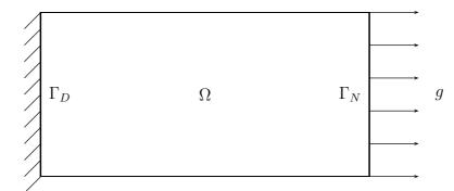
Figure 2: Geometry and problem description of Example 1.
