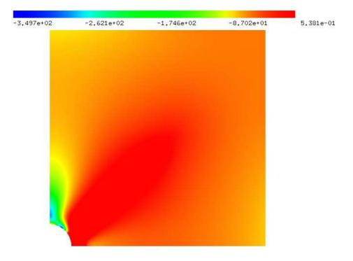
Figure 38: Yield function  $\phi$  (8) in Example 3.
