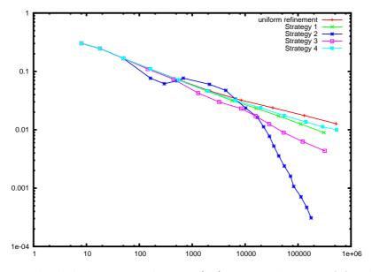
Figure 17: The global estimated error (45) versus degrees of freedom in Example 1.
