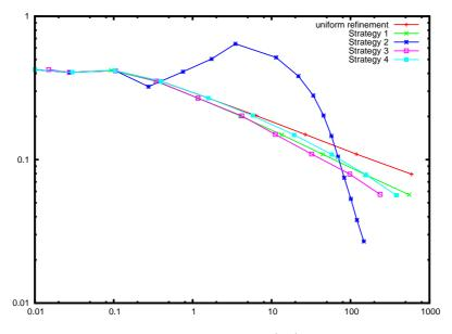
Figure 35: Here, the global estimated error (45) is plotted versus the time (in seconds) which was spent per Newton step in Example 2. One Newton step covers the assembling of the stiffness matrix and a sparse direct solver (PARDISO).
