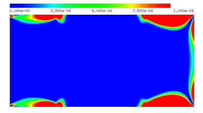
Figure 23: Frobenius norm of the plastic strain in Example 2.
