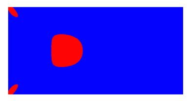
Figure 5: Plastic (red) and elastic (blue) zones in Example 1.
