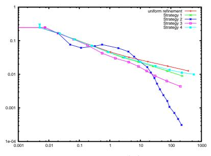
Figure 18: Here, the global estimated error (45) is plotted versus the time (in seconds) which was spent per Newton step in Example 1. One Newton step covers the assembling of the stiffness matrix and a sparse direct solver (PARDISO).
