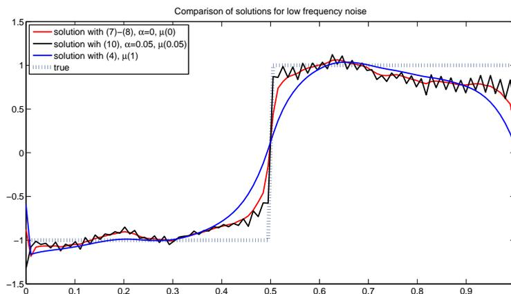
Figure 4: Comparison of solutions for the mildly ill-posed integration problem, 5% relative low frequency noise (cf. Figure 3) in the data,  $\mu$  according to (21),  $\tau = 1.1$ . The solution of the fractional methods (7)-(8) (solid) and (10) (dashed) with appropriate  $\alpha$  approximate the discontinuity much better than the results of Tikhonov regularization in standard form (dash-dotted).
