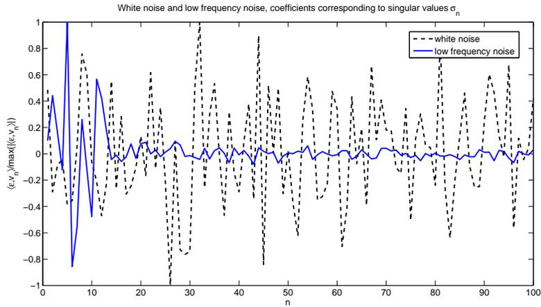
Figure 3: Comparison of typical random draws of white noise and low frequency noise w.r.t. the singular values. For white noise, the coefficients are equally distributed over all singular values. The low frequency noise decreases with growing  $n$ .
