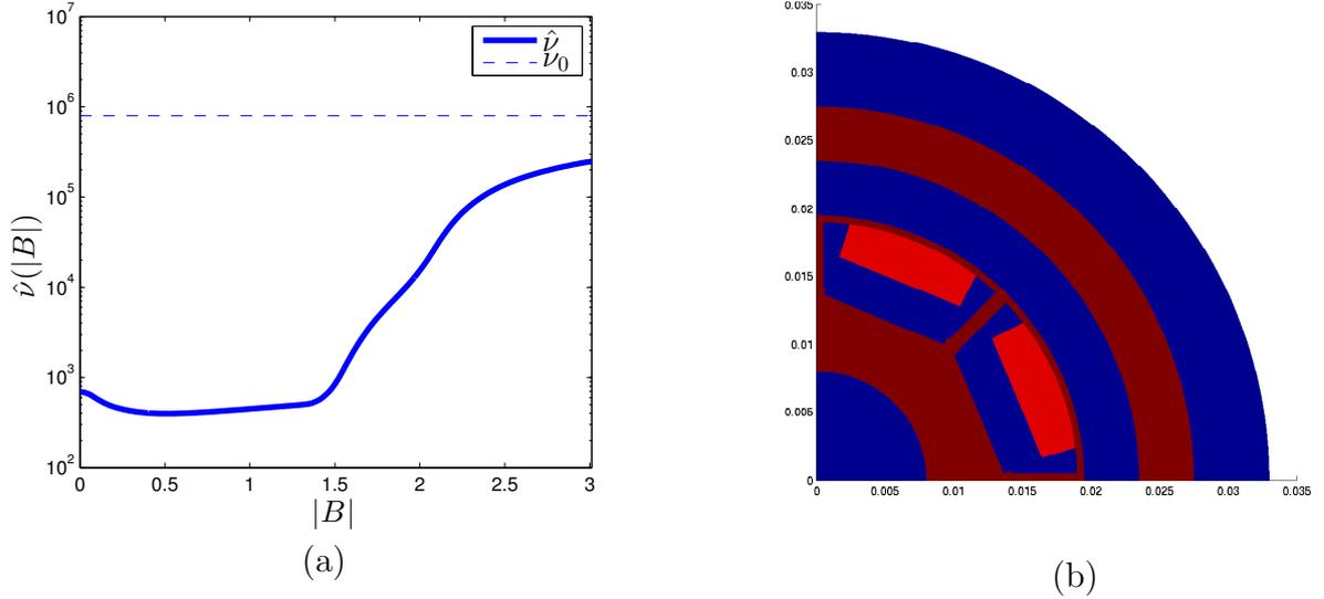
Figure 2: (a) Magnetic reluctivity  $\hat{\nu}$  as a function of the magnitude  $|B| = |\nabla u|$  of the magnetic flux density. (b) Ferromagnetic material  $\Omega_f$  with design subdomains  $\Omega \subset \Omega_f$  (highlighted).
