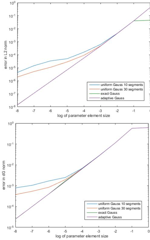
**Fig. 6.** Influence of the quadrature rule. Left: Convergence behavior of the error in L2 norm. Right: Convergence behavior of the error in dG norm. Blue and red curves: 10 and 30 uniform segments per  $t$ -knot span. Yellow curves: exact splitting of the knot spans. Purple curves: adaptive quadrature. Note that the yellow curve coincides with the purple one for smaller values of  $h$ . Exact representation of the reparameterizations  $\lambda$  and  $\varrho$ .
