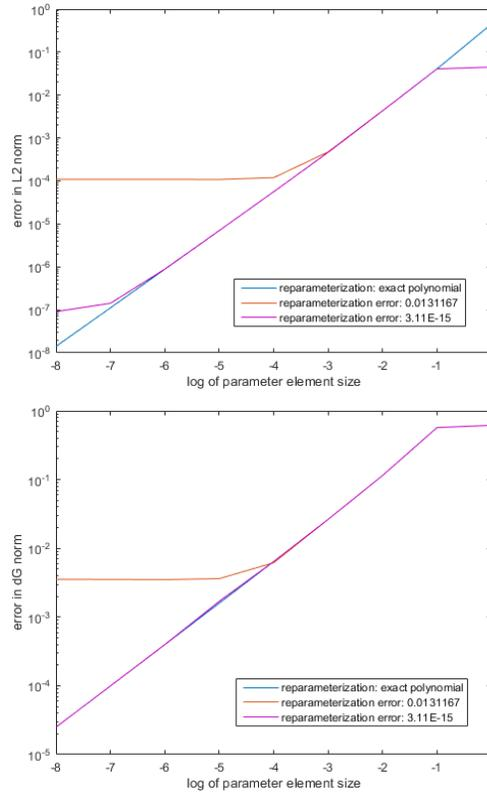
**Fig. 7.** Influence of the reparameterization. Adaptive quadrature on interface integrals. Left: Convergence behaviour of the error in L2 norm. Right: Convergence behaviour of the error in dG norm. Blue curves: Exact representation of  $\lambda$  and  $\varrho$ . Red curves: Approximation error of  $\varrho \approx 0.0131167$ . Yellow curves: Approximation error of  $\varrho \approx 3.10616 \cdot 10^{-15}$
