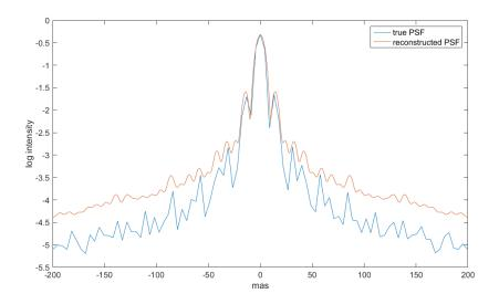
Figure 2: Zoom to the center of the true PSF (blue) and the reconstructed PSF (red) for  $n_{ph} = 1000$ , cut through the main diagonal.
