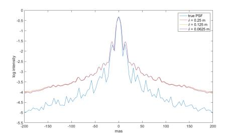
Figure 9: Zoom to the center of the comparison of the true PSF (blue) and the reconstructed PSF with a 2D structure function for  $\delta x = 0.25 \ m$  (red),  $\delta x = 0.125 \ m$  (yellow) and  $\delta x = 0.0625 \ m$  (purple) for  $n_{ph} = 100$ , cut through the main diagonal.
