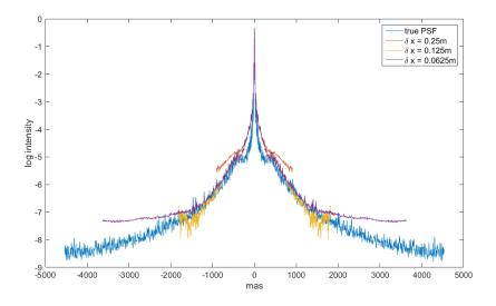
Figure 3: Comparison of the true PSF (blue), the reconstructed PSF with  $\delta x = 0.25 \ m$  (red),  $\delta x = 0.125 \ m$  (yellow) and  $\delta x = 0.0625 \ m$  (purple) for  $n_{ph} = 1000$ , cut through the main diagonal.
