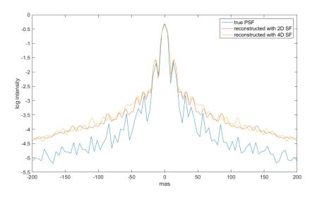
Figure 6: Zoom to the center of the comparison of the true PSF (blue), the reconstructed PSF with  $\delta x = 0.25 \ m$  using a 2D structure function (red) and a 4D structure function (yellow) for  $n_{ph} = 1000$ , cut through the main diagonal.
