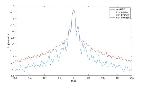
Figure 7: Zoom to the center of the comparison of the true PSF (blue), the reconstructed PSF using the 4D structure function with  $\delta x = 0.25 \ m$  (red),  $\delta x = 0.125 \ m$  (yellow) and  $\delta x = 0.0625 \ m$  (purple) for  $n_{ph} = 1000$ , cut through the main diagonal.
