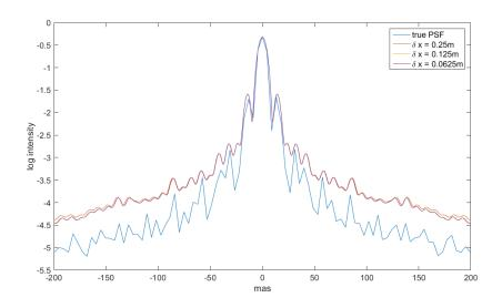
Figure 4: Zoom to the center of the comparison of the true PSF (blue), the reconstructed PSF with  $\delta x = 0.25 \ m$  (red),  $\delta x = 0.125 \ m$  (yellow) and  $\delta x = 0.0625 \ m$  (purple) for  $n_{ph} = 1000$ , cut through the main diagonal.
