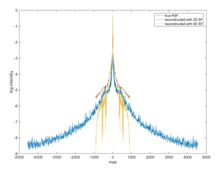
Figure 5: Comparison of the true PSF (blue), the reconstructed PSF with a 2D structure function (red) and 4D structure function (yellow) for  $n_{ph} = 1000$ , cut through the main diagonal.
