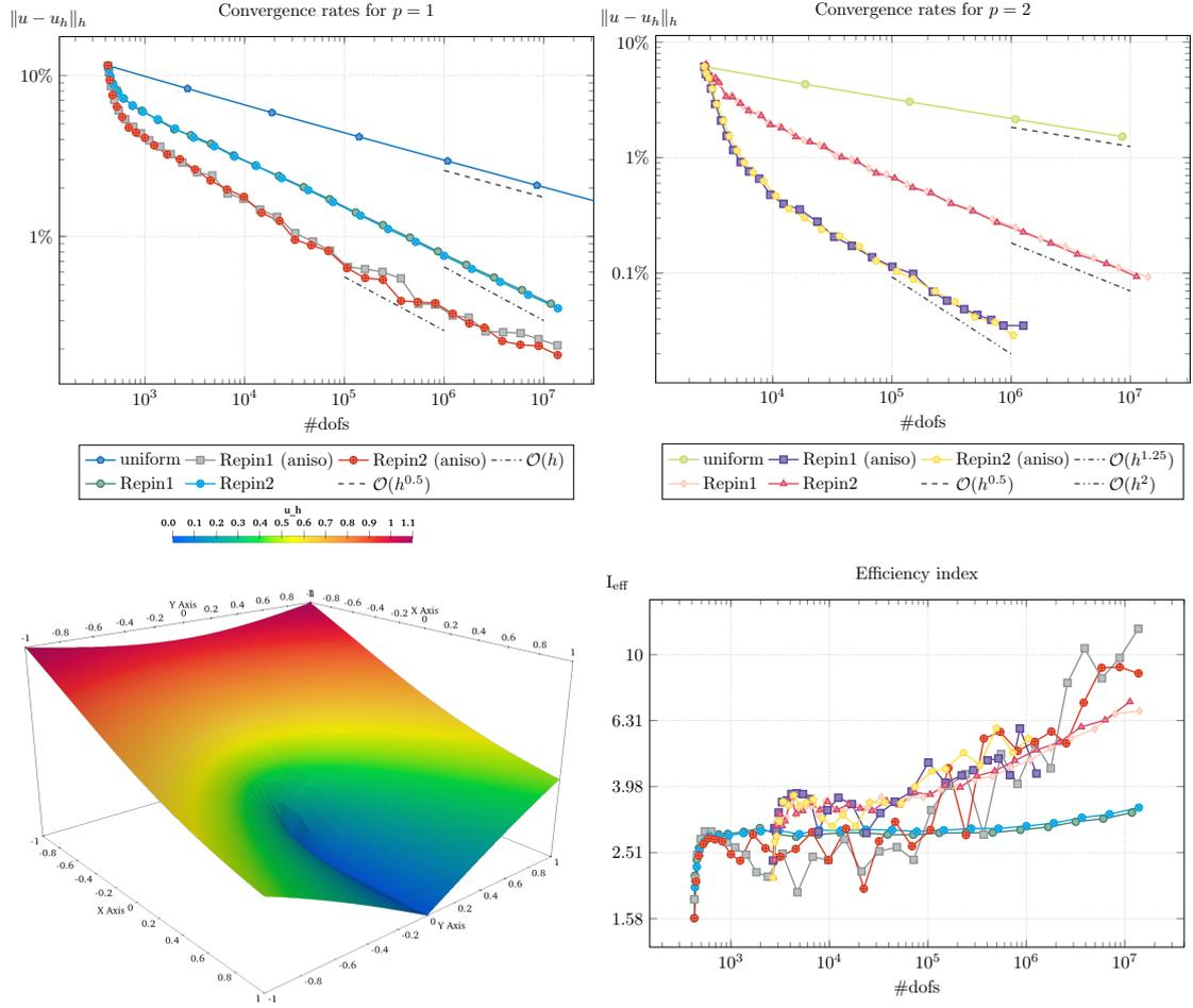
**Fig. 1:** Convergence rates for  $p = 1$  (upper left); convergence rates for  $p = 2$  (upper right); plot of  $u(\cdot, \cdot, 1)$  (lower left); efficiency indices for  $p = 1, 2$ , with the respective colors from the upper plots (lower right).
