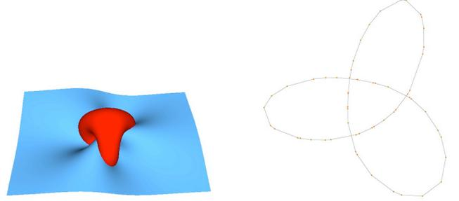
**Figure 5: Piecewise linear approximation of the trefoil knot, computed as the intersection of two implicit surfaces with algorithm APPROXLINK in Axel**
