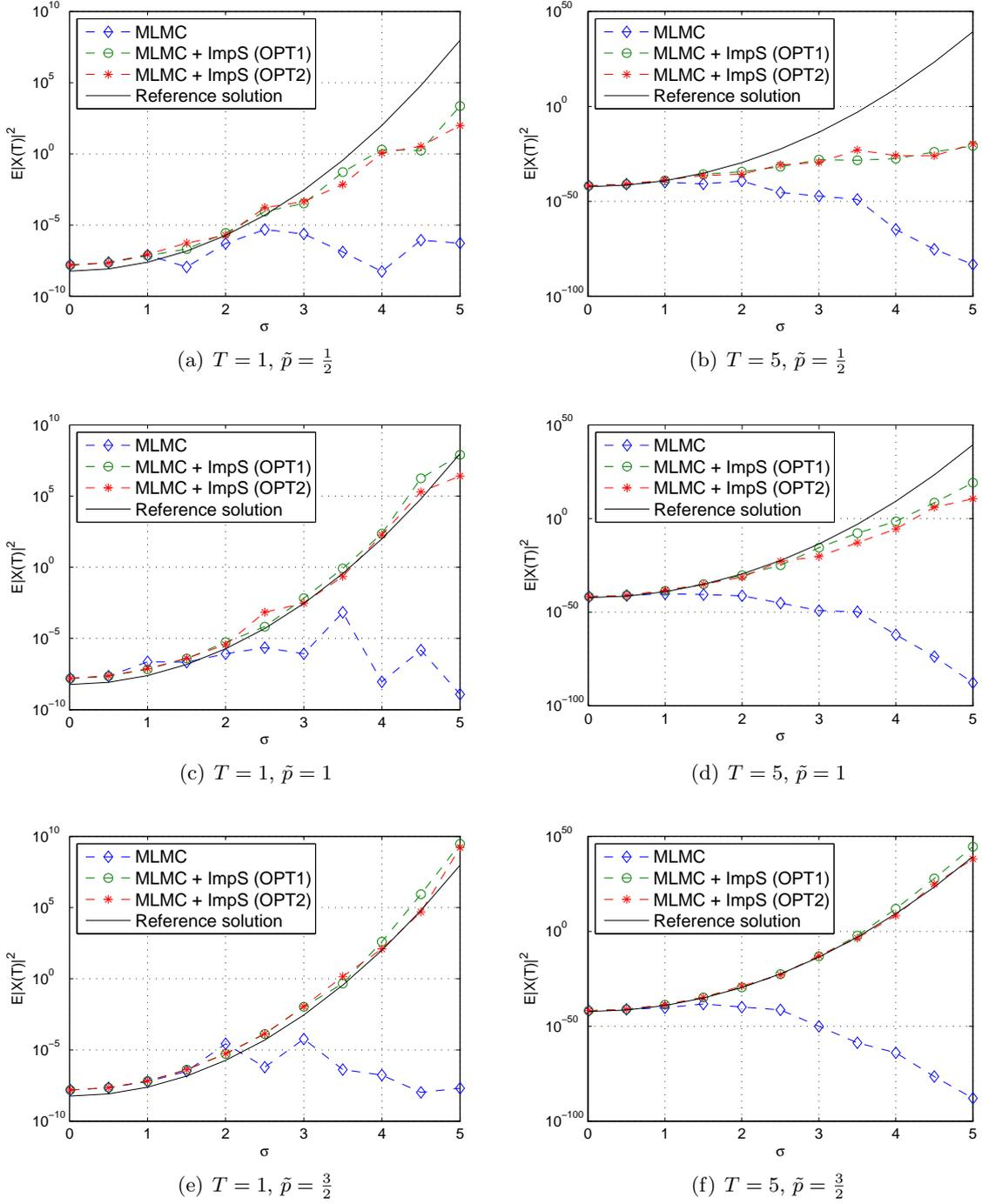
FIGURE 3. Multilevel Monte Carlo methods for the spatially discretised stochastic heat equation (8) for  $N = 10$  and varying  $\sigma$ . The reference solution is computed by Eq. (21).
