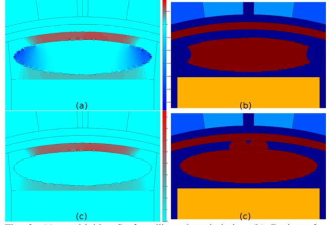
Fig. 2. (a) sensitivities  $S_k$  for ellipse-shaped design (b) Design after removing material according to sensitivities  $S_k$ ,  $J(u) = 0.436$  (c) generalized topological derivative for ellipse-shaped design (d) design after adding material according to topological derivative,  $J(u) = 0.406$
