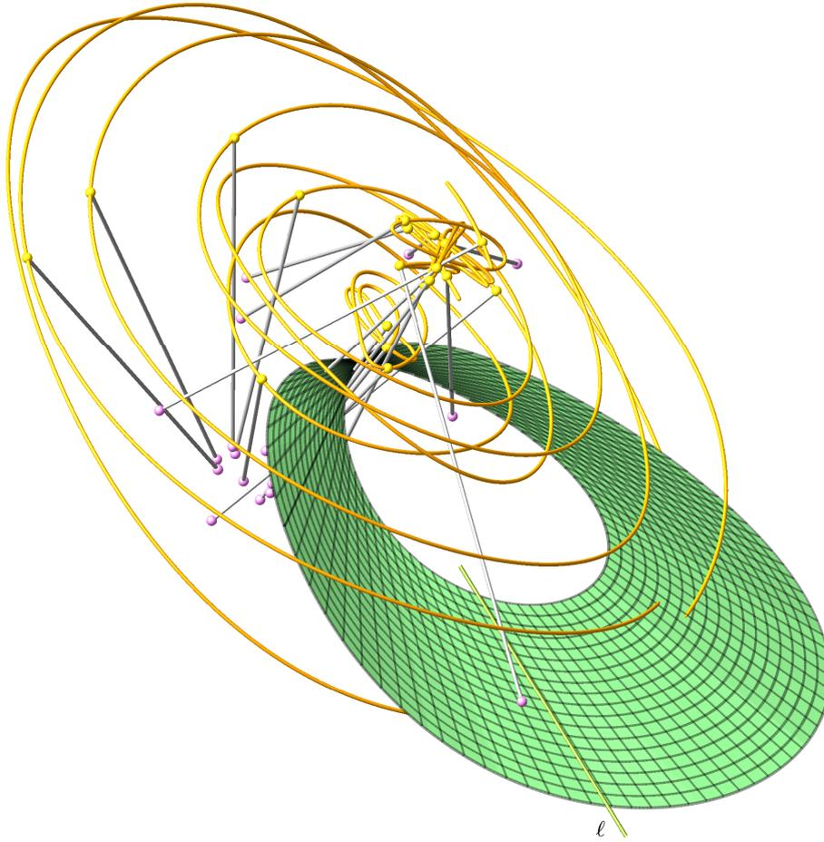
FIGURE 4. The same set-up as in Figure 3 but from another perspective. In addition a strip of the base surface of this line-symmetric self-motion is illustrated, where  $\ell$  is highlighted. Note that one of the two displayed families of curves on the surface is composed of straight lines, i.e. the generators of the ruled surface.
