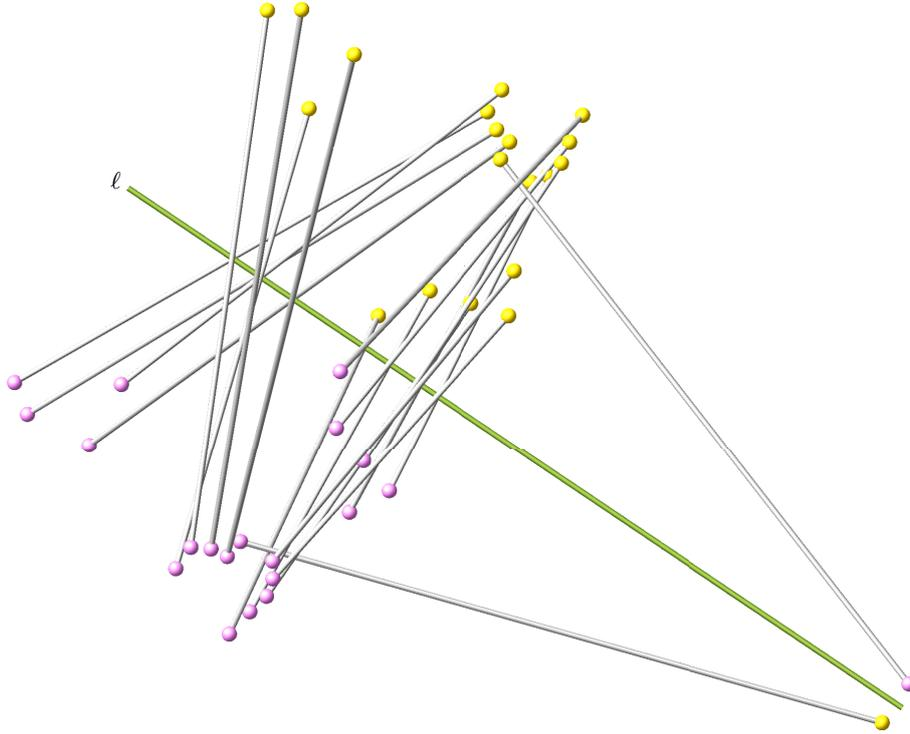
FIGURE 1. Base points (pink) and platform points (yellow) of an icosapod. Notice that for every leg there is a symmetric one obtained by rotating the first one by  $180^\circ$  around the axis  $\ell$ . The symmetry reverses the role of base and platform points.
