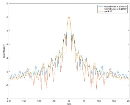
Figure 6: Zoom to the center of the comparison of the true PSF (yellow) and the reconstructed PSF with 4D structure function (blue) and 2D structure function (red) for  $n_{ph} = 100$ , cut through the main diagonal.
