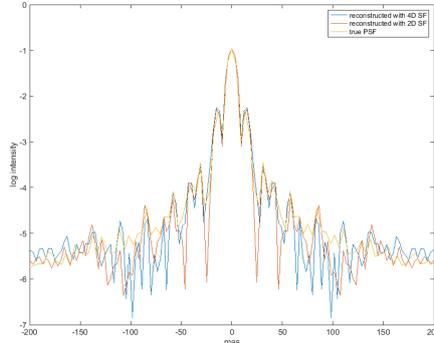
Figure 4: Zoom to the center of the comparison of the true PSF (yellow), the reconstructed PSF using a 2D structure function (red) and a 4D structure function (blue) for  $n_{ph} = 1000$ , cut through the main diagonal.
