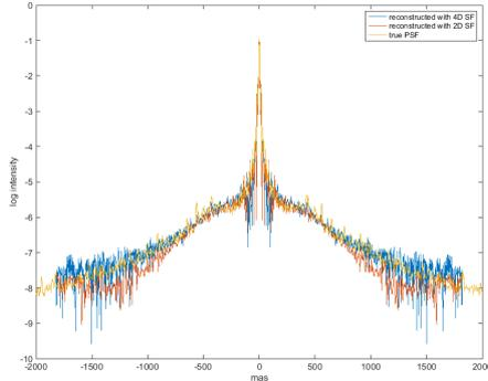
Figure 3: Comparison of the true PSF (yellow), the reconstructed PSF with a 2D structure function (red) and 4D structure function (blue) for  $n_{ph} = 1000$ , cut through the main diagonal.
