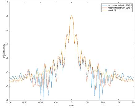
Figure 5: Zoom to the center of the comparison of the true PSF (yellow) and the reconstructed PSF with 4D structure function (blue) and 2D structure function (red) for  $n_{ph} = 500$ , cut through the main diagonal.
