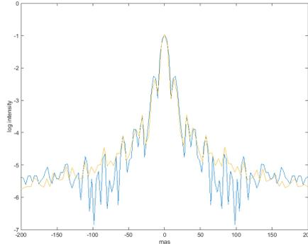
Figure 2: Zoom to the center of the true PSF (yellow) and the reconstructed PSF (blue) for  $n_{ph} = 1000$ , cut through the main diagonal.
