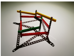
Fig. 1. Here is an L-model of a moving graph K_{3,3} . The edges correspond to sticks with holes, and the vertices correspond to gray columns.
